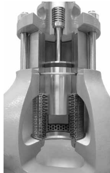
Figure 1. Typical Valve with WhisperFlo Aerodynamic Trim
