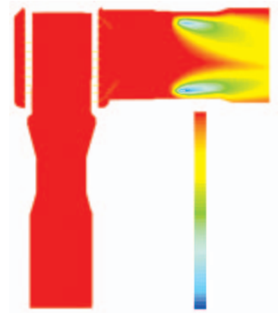
AF nozzle spray atomization under Computational Fluid Dynamics (CFD) analysis
