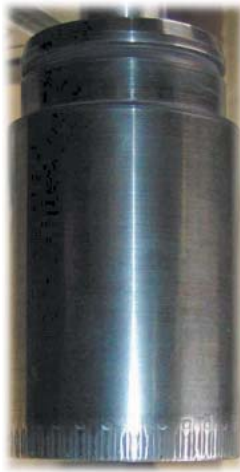
Figure 1. Anti-cavitation trim valve plug showing low-flow erosion damage. Photo courtesy of Fisher Controls International, LLC.
