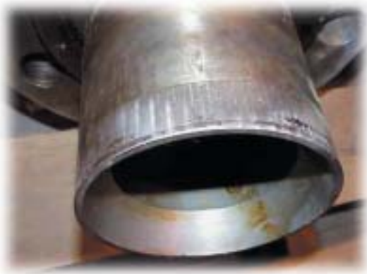
Figure 2. In detail, erosion and cavitation damage due to low-flow erosion. Photo courtesy of Fisher Controls International, LLC.
