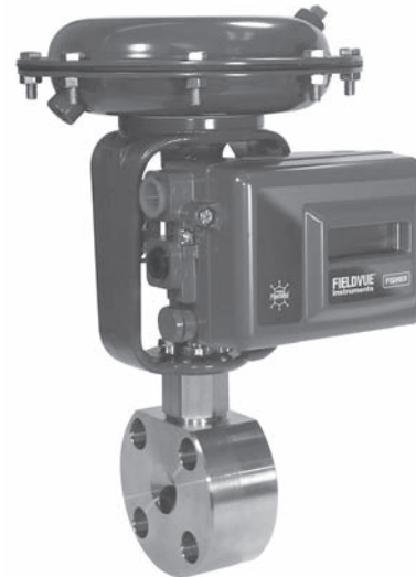
Figure 2. 24000F Control Valve with Baumann 32 Actuator and FIELDVUE DVC2000 Digital Valve Controller
