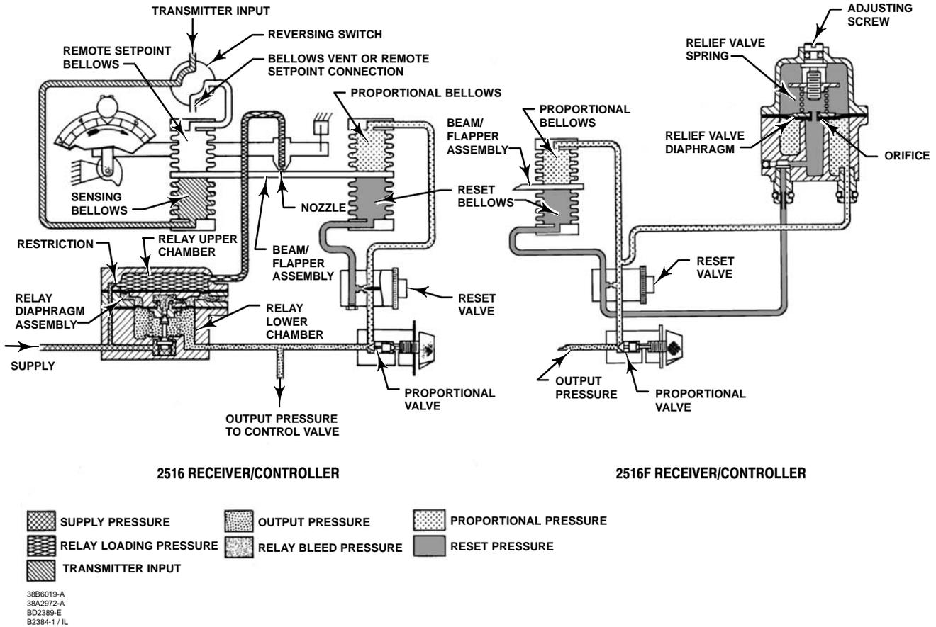
Figure 5. 2516 Receiver-Controller Schematic
