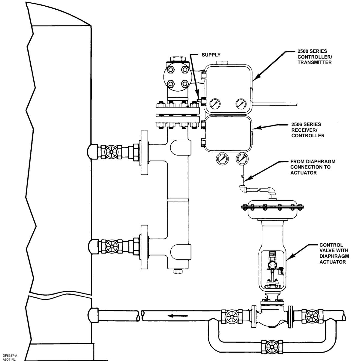
Figure 6. Receiver-Controller Mounted on a 2500 Series Controller/Transmitter
