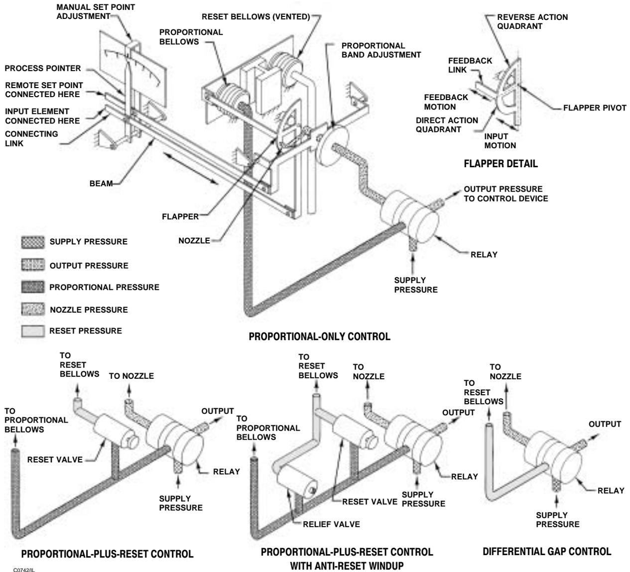
Figure 2. Operational Schematic of 4194 Series Differential Pressure Controllers
