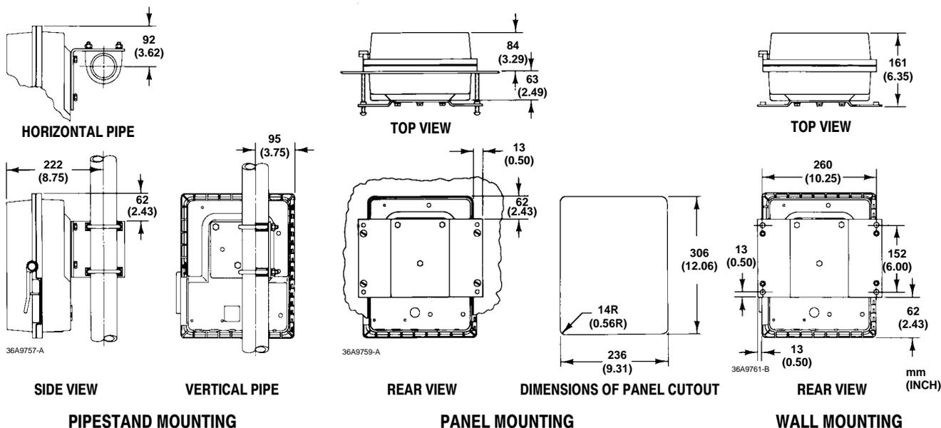
Figure 6. Mounting Dimensions
