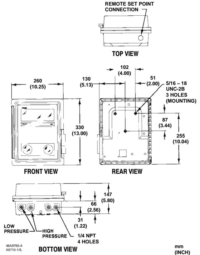
Figure 5. Controller Dimensions
