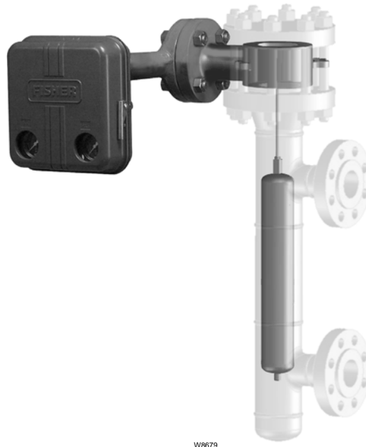
Figure 4. L3 Pneumatic Level Controller (2500 Controller in Combination with a 249W Sensor)— Installed in a Typical Customer-Supplied Cage
