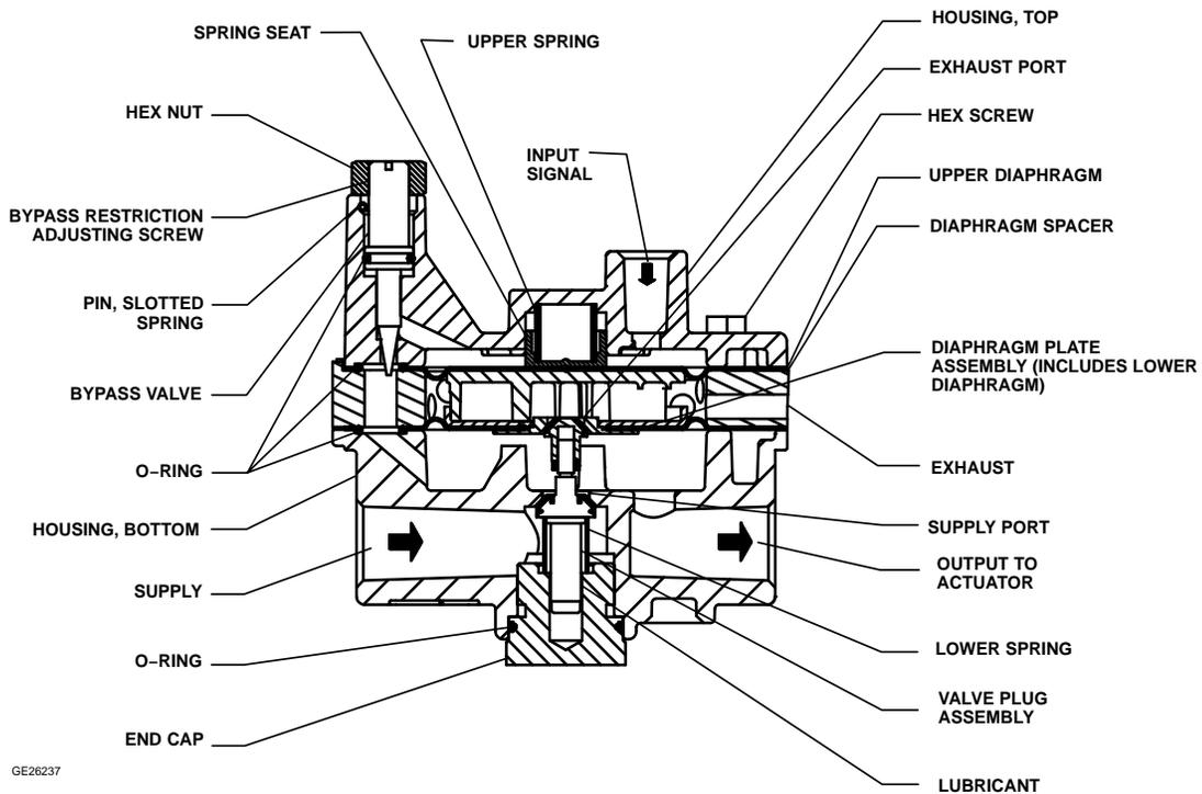
Figure 2. Volume Booster Sectional View
